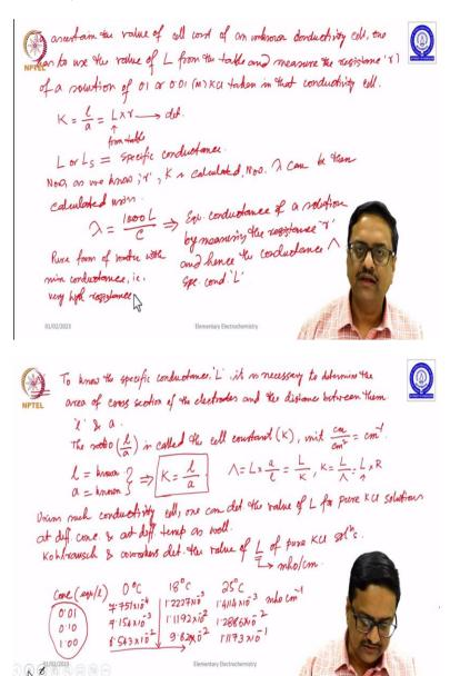
So, to ascertain the value of cell constant of an unknown conductivity cell one has to use the value of L from the table and measure the resistance say small r of a solution of 0.1 or 0.01 molar kcl taken in that conductivity cell. So, this cell constant K is nothing, but l by a which is equal to L into r which we have shown in the previous picture that is L into r. So, this value of L from table and r is determined using the Wheatstone bridge principle.
