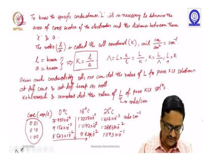
So, what we have determined is we have obtained the value of lambda, but to know the specific conductance that is capital L it is necessary to determine the area of cross section of the electrodes and the distance between them that is l and a. The ratio l by a is called the cell constant. So, what will be the cell constant which is written as capital K, what will be the unit of cell constant?
