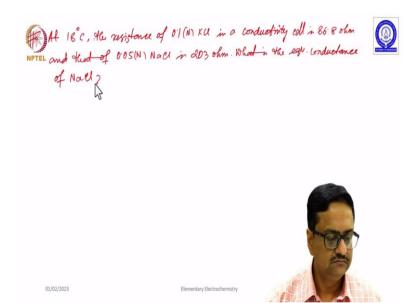
So, before we end today's class I would like to give you one problem to solve. The problem is at 18 degree centigrade the resistance of 0.1 normal K cl is in a conductivity cell is 86.8 ohms and that of 0.05 normal NaCl is 203 ohm. What is the equivalent conductance of NaCl? So, you will need the value of specific conductance of K cl solutions at 18 degree centigrade from the table and then you try to solve this problem. We will continue from here in the next class. Thank you.
