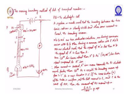
So, this is called the moving boundary method of determination of transport number. So, in this method we will be using a different type of an electrochemical setup which I am going to draw here and we will continuously explain what I am drawing. I have a glass tube which is reasonably long glass tube with two ends fact like this for the introduction of the corresponding electrodes.
