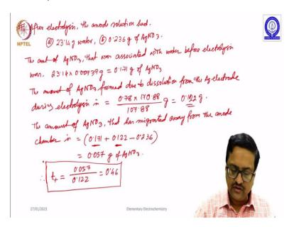
So, in the problem we said that after electrolysis the anode solution had number a 23.14 gram water and 0.236 gram of Ag NO3. Now we can calculate that the amount of Ag NO3 that was associated with water before electrolysis was 23.14 into 0.00739 gram or equal to 0.171 gram of Ag NO3. Now the amount of Ag NO3 formed due to dissolution from the Ag electrode during electrolysis is equal to 0.78 into 170.88 divided by 107.88 gram or simply equal to 0.122 gram.
