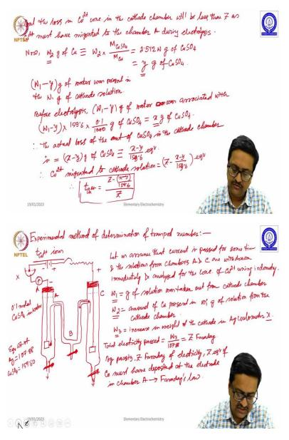
But the loss in CO 2 plus concentration in the cathode chamber will be less than z as CO 2 plus must have migrated to the chamber A during electrolysis. Now w 2 gram of copper is equivalent to w 2 into M Cu SO 4 by M Cu that is molecular weight of copper sulphide by molecular weight of copper is equal to 2.512 w gram of Cu SO 4 which we write as y gram of Cu SO 4.
