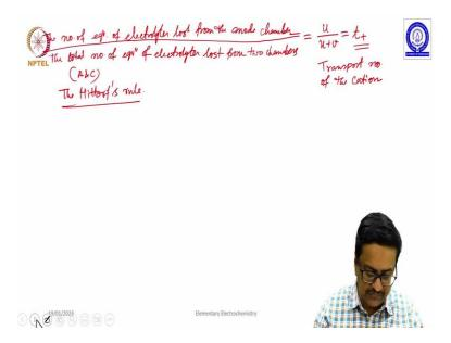
So, one can write that the number of equivalents of electrolytes lost from the anode chamber divided by the total number of equivalents of electrolytes lost from two compartments or chambers A and C together is equal to u by u plus v which is nothing but what we learned in the previous class is t plus the transport number of the cation.
