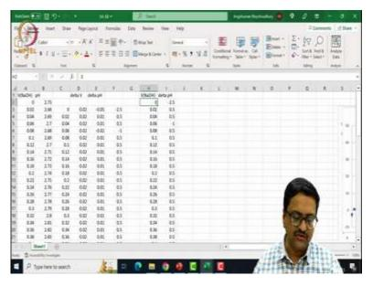
What you are seeing here in this screen is the volume of NaOH that is marked 0 and we started at 2.73 value of pH. And then we continued adding small, small fractions 0.02, 0.06, 0.08 that means every time we are adding 0.02 ml of NaOH and we noted down the corresponding value for the pH. And if you remember we have done it till the pH reached 10.67.
