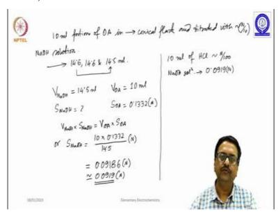
So, after that what we had done is we had taken 10 ml portions of oxalic acid in a conical flask and titrated with approximately N by 10 NaOH solution. So, during that titration when we had done the titration three times, we got the readings as 14.5, 14.6 and 14.5 ml in three consecutive titrations.
