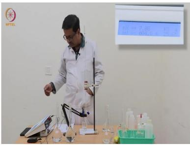
Now, by stepwise addition, I have reached a point where I have added 1.30 ml and the pH reads 5.38 which now indicates that the S type of curve has started going upwards. So, to draw a curve very nicely, one should have readings with very small valid difference in the volume of NaOH added that is, we should now use again 0.2 ml steps at a time. So, with just addition of 0.02 ml of this NaOH which is 10 times stronger has increased the pH from 5.38 to 5.83.
