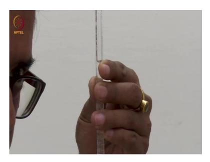
So, now in this third experiment, I am going to use a weak dibasic acid, which is here, this is oxalic acid dihydrate approximately N by 100 strengths. As usual, this is a very dilute solution of approximate and by 100 concentrations. And I am going to titrate this using the standardized N by 10 Approximately N by 10 NaOH solution. So, this NaOH solution is 10 times more concentrated with respect to that oxalic acid.
