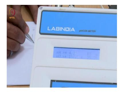
So, now we are at 0.72 and the pH has changed to 3.67 which is like 0.08 in terms of pH. Now, we have reached 0.74 and pH is 3.72. So, we have just re crossed the half equivalence point and then we should continue as usual till we see a jump above pH 7, which will indicate the complete neutralization point. Now we have reached a point of 0.90 ml that is now the pH is 4.09 where we can see that again the pH is starting to increase because we are now nearing the complete equivalence point.
