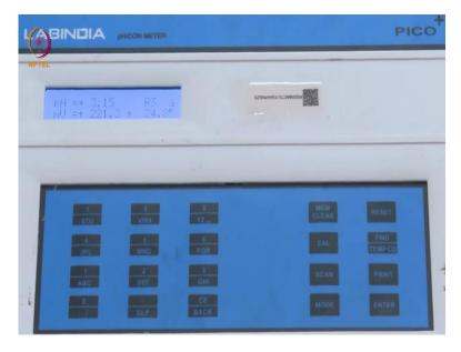
So, after addition of 0.02 ml of NaOH the pH has not changed much it remains that 2.68 So, we should continue this addition as before which we have already done for strong acid and strong base and then for weak acid and strong base. So, with the addition of 0.04 ml of NaOH now the pH has slightly increased to 2.83. So, we will continue to add as before 0.02 ml further of.
