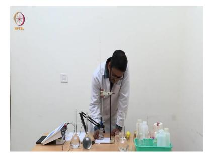
So, this time I am using a different pipette pump, which you can see here in my hand. So, we will use this different type of pipette pump to pipette out 10 ml of HCl. And we carefully take it only up to the mark which indicates 10 ml, we have a mark here in the pipette, as you may be able to see the mark is at this point here, which indicates that we have 10 ml solution in the pipette.
