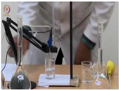
So, that we reach the equilibrium and the stable pH is red. So, it is with 0.4 ML the rating is 2.69 you must appreciate that this pH is not changing because this is strong acid which is completely dissociated in solution and hence the pH does not change with addition of NaOH significantly from the burette. So, I am going to continue this edition of NaOH very little at a time and every time I have added 0.2 ML, which means now I have added 0.6 ml and reading still 2.69.
