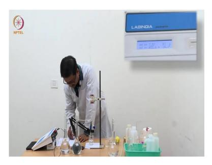
So, we should take the reading when it stabilizes the pH. Maybe 5.57 then we add again 0.02 ml and reach 1.2 ML the pH comes out comes about 5.7476. So, it takes a while to stabilize. So, with addition of 1.2 ML the pH is 5.83. So, now with 1.24 ML the pH has come almost to the neutral pH of water it is about 6.73.
