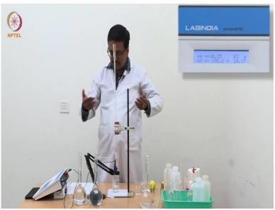
So, now, what you can see is with addition of 1.30 ML the pH has jumped up to 8.64 as you can see in your screen, which essentially means, we have crossed the equivalence point we will need about 3 to 4 points beyond this for a good pH curve that I have shown you in the class by hand drawing with this experiment we can achieve that kind of curves as well we experimental curve can we achieve.
