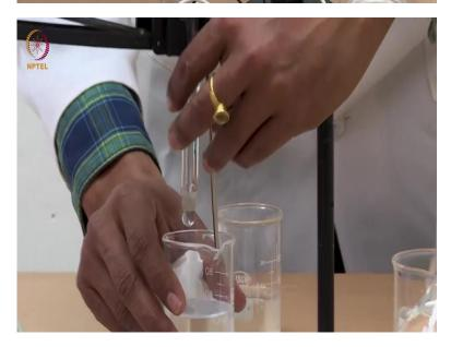
So, now we are here ready with the setup with a pH conductivity meter SpH cum conductivity meter which you can see in your screen, this pH conductivity meter has two options with a pH electrode which will measure the EMF change inside the solution and convert it into the corresponding value of pH is now connected and this pH conductivity meter when it is running in the PH mode, we need to do a calibration.
