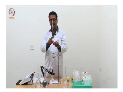
So, what you can see that in the beginning the pH was not changing towards the equivalent point the pH was changing slowly near the equivalence point the pH changed drastically close to 7 and then it has reached 8, 9 and 10 And now, with addition of more amount of NaOH, the pH is not increasing significantly as it was doing when the equivalence point was reaching.
