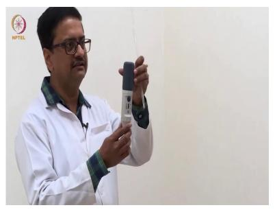
So, for acid base titration, we use normally the oxalic acid dihydrate which is here in this bottle, this is a particular type of bottle we call it as the weighing bottle, you can see that we have the groove here and the lid and this comes in pair. So, when you have the bottle and the lid proper and then you take oxalic acid in this, we will use this weighing bottle to do the weighing.
