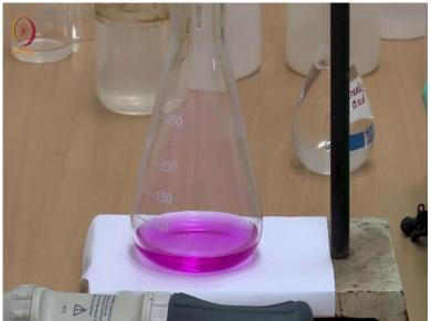
So, for this acid base titration using NaOH as the titrant and oxalic acid as a primary standard. We need to use phenolphthalein solution as indicator you know phenolphthalein is a colourless solution in acidic medium, but in alkaline medium, it will change its colour to a bright pink colour. So that will indicate the endpoint of this reaction.
