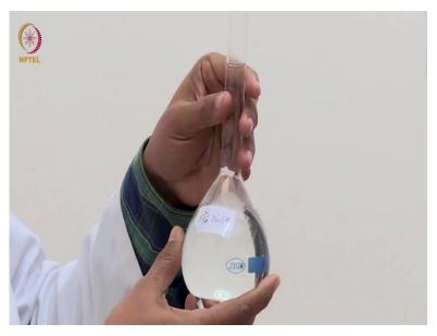
So, I am now taking out this bottle from here and carefully trying to transfer a very small amount by not moving the lead completely away, but carefully transferring tiny amounts of oxalic acid in the volumetric flask and then taking it down and we will place it back to the balance and what I see here is it is reading 34.22. That means we have not transferred enough amount of oxalic acid.
