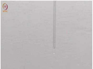
So, at the beginning we need to standardize this NaOH for our next set of experiments. So, we will do this standardization using a 250 ml conical, where we will be pipette out our oxalic acid and we will use this 50 ml burette which I have already mounted on this stand and clamp. We will Use this burette and fill it with sodium hydroxide and do the titration. Maybe it is better to keep a thing if there is a leakage it will fall on that only.
