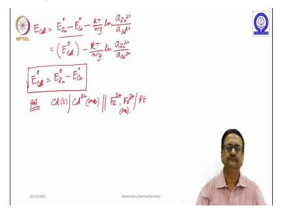
So, what one can simplify from here is that E cell equal to E0 Z n minus E zero copper minus RT by nF ln activity of Zn 2 plus divided by activity of co2 plus. Therefore, these two can be replaced by E0 cell minus R T by nF ln activity of Z n 2 plus divided by activity of Cu 2 plus. So, what does it mean, we can easily write E0 cell is equal to E0 Z n minus E0 of copper. So, with this one can very easily calculate the standard emf of a given cell.
