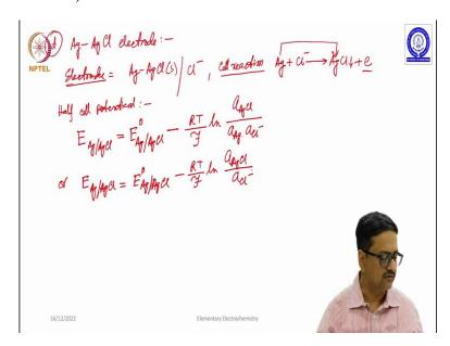
So, we also learned about the silver silver chloride electrode in the previous lectures. So, we should also try to write down the same equation for Ag, AgCl electrode. So, what is the electrode here, the electrode is Ag in connection with AgCl in solid and in equilibrium chloride ions in solution.
