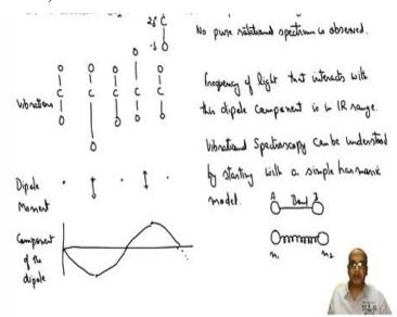
It will look like so the dipole is 0 over here, so these are vibrations and the dipole moment looks like this. So, dipole moment is zero here; I can say that the direction is downward here zero here again direction of the dipole is upwards, zero here again. So, again, it is following up periodic motion, if you look at the vertical component of the dipole moment. So, I can say the component of the dipole, so it will be 0 at this point, then negative at this point, zero again, positive, 0.
