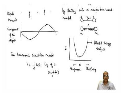
Now all of this will change the energy of this system, so how do I describe this change in energy? I can always say that if I plot energy here, and let us call the mean distance as r, r here. So, at the equilibrium distance, the energy will be minimum. Now, as I start to stretch the bond length will increase, so this is my bond length and the energy will increase so it will go like this. Now, as I start to compress again the energy will increase, it will go like this.
