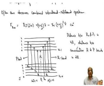
Now, we can always calculate now the delta E between different levels between different J levels and different v levels. So, now let us look at a transition between v equal to 0 to v equal to 1, so for every vibrational level there are some rotational levels, because at each vibrational state a molecule is rotating, so those rotational levels will correspond to that particular v. So, let us say this v equal to 0 and v equal to 1, so at this we I will have different J levels like this.
