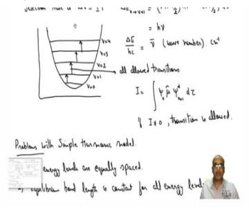
So, this is basically called as simple harmonic model but there are problems with simple harmonic models, so what are the problems? Let us discuss that problem with simple harmonic model. So, first of all, it defines that all energy levels; all energy levels are equally spaced. That means all the spectral lines will come at exact same position in frequency but you do not see that you do see multiple lines.
