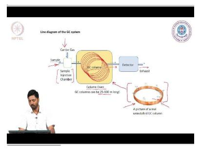
Now, let us move forward and see a very basic line diagram of a gas chromatography system. So, we inject our sample from one side of this chromatographic system and we also pass in the carrier gas into chromatographic system, these 2 mix in what is known as the sample injection chamber. So, the vaporize sample or the sample vapors and the carrier gas mix together in sample injection chamber.
