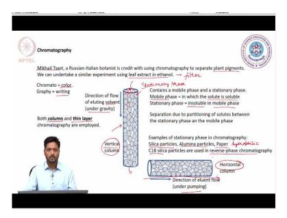
So, let us go to the slide and understand what do we mean by chromatography. So, chromatography as the term indicates it is literally meaning chromatic which is color and graphy which is writing. So it is some sort of mark or writing that occurs when analytes are separated especially analytes, which are colored and Mikhail Tsvet is Russian Italian botanist who is credited with having used chromatographic techniques to separate plant pigments.
