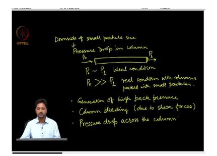
Another very important downside of having small particle size is that we create what is known as the pressure drop in the column. So, if we are talking about a long column and we are applying pressure P 0 here and we are measuring the pressure that is at the other end of the column let us call it as pressure P 1, what we would ideally want is that the P 0 is similar to P 1.
