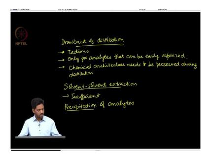
So, to mention the drawback of distillation we observe that it is of course a tedious process and is amenable only for solids or analytes that can be easily vaporized. Now, it is of course true that not very many organic compounds can be easily vaporized while ensuring the chemical architecture. So, the chemical architecture needs to be preserved during distillation and that started becoming a challenging process for a large number of solids.
