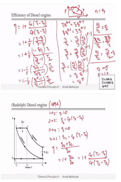
So efficiency Eta is 1 plus C V T 1 minus T 4 C P T 3 minus T 2. Now we know that C P by C V is gamma, so it is 1 by gamma T 1 minus T 4 and T 3 minus T 2. Now let us simplify this process and I am going to draw it here just for remembering this is a constant pressure process so 1, 2, 3 and 4 these are two adiabatic processes and this is a constant pressure process is constant volume process just to remember that this is a handy way to have that.
