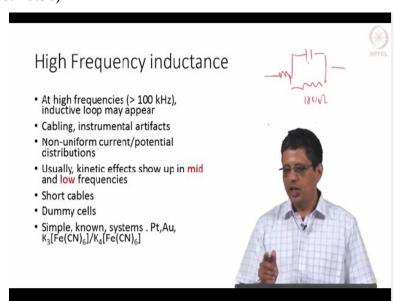
Usually the kinetic and mass transfer effect will show up at the middle and low frequencies. If you have doubt about the results, what you should do is first take a dummy cell. Dummy cell
