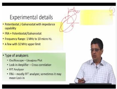
In the oscilloscope, at a given frequency, you will apply a potential, sinusoidal potential; You will also get current, It may have a phase difference. And you would actually plot potential and current as a function of time. It may go like this, it may go like this and there will be a point
