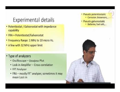
So if I give 10 mV potential and let us say the magnitude of the impedance is 1 m $\Omega$ . the current that I get is going to be, [this many volts by ohms, would give me ] 10 A current. On the other hand, instrument can give a constant current or a small oscillation in the current, it can measure the potential very accurately. So here if I give 100 mA current, that means 0.1, I would get  $10^{-4}$ , that means 0.1 mV at the peak.
