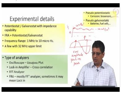
This term FRA is a *frequency response analyzer*, most of the times, it means *it is an FFT analyzer*, although I think sometimes it is being used for instrument which also use cross correlation. If you remember right, one of the vendor, Solectron uses cross correlation and call that equipment as an FRA, frequency response analyzer. And of course, most of the manufacturers will not even tell you how they actually analyze the data, and give you this result.
