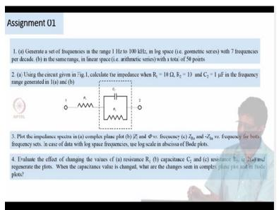
So I want to describe the assignments. In this assignment, first I want you to generate a set of frequencies, in both log scale as well as in linear scale. The idea is this: if you have an electrical circuit and you measure impedance spectrum, then if the frequencies are in log scale, what would you see; and if the frequencies are in linear scale, what will we see. So for that I have split that into multiple questions.
