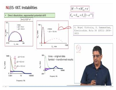
Next, okay we know how to generate the spectrum incorporating the instability effects or drifts, we seen this in the previous class, so I want to show you an example where we have taken the simple electron transfer reaction and we apply an exponential drift, okay, this is published in 2011 by our group and we have seen before that if you have 10 millivolts or 100 millivolts drift, maximum possible drift with a particular b value, this is the data that you would get.
