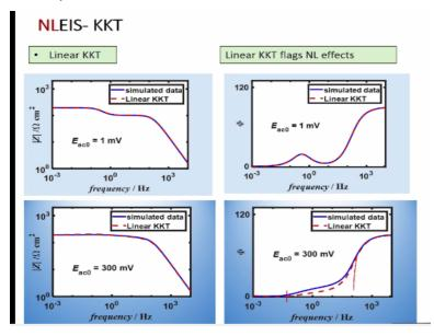
When you use a linear KKT software and compare the transformed data and the original data, they overlap very well for 1 millivolt data and at 300 millivolt, there is a difference especially at the mid frequencies, the magnitude appears to overlap very well, the phase is different which basically tells you that there is a difference between the original data and the transformed data, so it is not KKT compliance.
