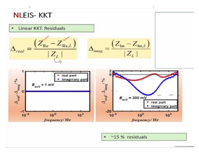
In case of linear KKT software, it is also good to look at the residuals, this also flags the nonlinear effect but one can calculate the residuals; the residual in the real values are basically, our simulation or original data minus the best fit, measurement model approach best fit data divide by the modulus of the Z, not Z real or Z imaginary but actual Z which is Z real + j Z imaginary.
