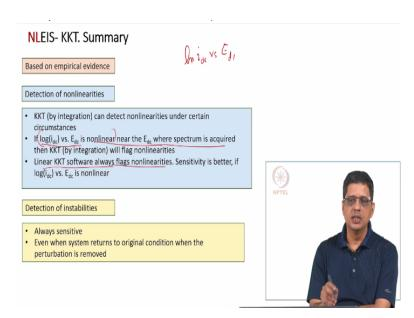
So, in summary, based on empirical evidence that means we are not shown theoretically that when log I versus E is a straight line, when it is linear, the violations of linearity will not be captured by KKT, KKT will not flag the spectrum acquired at large amplitude perturbations but with a number of simulations what we conclude is that if log I versus Edc is non-linear near the Edc where the spectrum is acquired.
