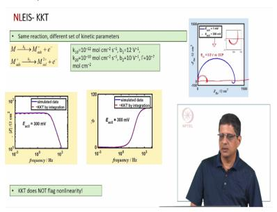
All right, now we have taken the same mechanism and tried different sets of kinetic parameters, different sets of DC potentials and in all cases, you would get spectra, we have tested many but we are showing a few here, okay, this is second example, same mechanism different set of kinetic parameters. Now, in this case we have taken the DC potential to be 0.5 volts versus OCP, we have tried 1 millivolt linear regime and 300 millivolt nonlinear regime.
