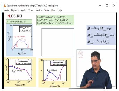
Next example is for a 3 step reaction to adsorb intermediates, so the mechanism we have seen this kinetic parameters we write it as 10 power -10, 15 for the first reaction, 3.3 10 power -12 and 20, 7 10 power -7 and of course third reaction is a chemical reaction, so there is no b corresponding to that and gamma is 10 power -7 moles per centimetre square. In this case, when we use 1 millivolt data, we get 2 semicircles.
