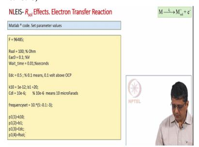
So as an example 100 ohm solution resistance Eac0 is 100 millivolt you can say (()) (15:51) is 10 milliseconds we apply a dc potential we set the kinetic parameters values and set the frequency range. We want to pass the kinetic parameter values as vector.
