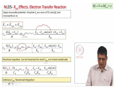
Now we have to visualize the E2 the potential drop across the interface as a sum of dc and ac but here I use the term ac in a loose fashion. It is not necessarily sinusoidal oscillation at frequency of omega. So you can write the equation instead of E2 you can write it as E2 dc+ E2 ac and this is what you would get. This is the potential that we apply a dc bias + an ac potential and that is at sinusoidal frequency omega we control that.
