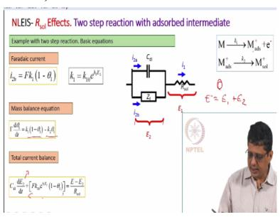
Now what happens when you have an intermediate species it is an example two step reaction with an adsorbed intermediate. So the same electrical circuit equivalent circuit the faradaic current I would write it as F k1 1-theta for this theta is the fractional surface coverage of the adsorbed intermediate and k1 is related to the potential as k10 b1 E2 it is not k10 b1E. Mass balance equation of course we are seeing this before it is gamma d theta 1/dt.
