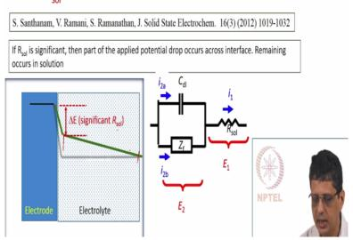
So some of this work we have published in 2012 this is a schematic, illustrating how the potential drops occurs this electrode, electrolyte interface if we have negligible solution resistance we can say that all the potential drop occurs across the interface and then we can model this with a circuit given here that is double layer capacitance being parallel with the faradaic impedance.
