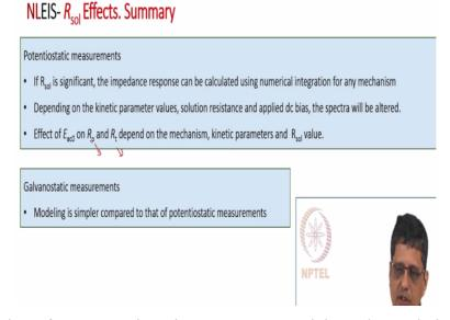
So all this is done for n potentiostatic measurements right. When solution resistance is significant you can calculate the impedance response using numerical method. You have to use integration for pretty much any mechanism and depending on the dc bias, depending on the kinetic parameter values, depending on the mechanism, depending on the solution resistance the measured spectrum or simulated spectrum will change.
