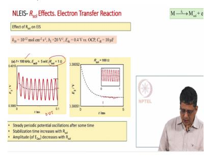
Now for a given set of kinetic parameter right if I apply a frequency of 100 kilohertz for a solution resistance of 1 ohm for a simple electron transfer reaction the potential oscillation stabilize after sometime. Earlier we have seen that when you have adsorbed intermediate the current oscillation will stabilize after sometime right.
