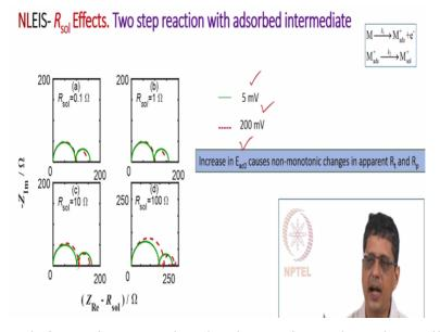
Now if I fix the solution resistance and replot that so that I plot only 5 millivolt and 200 millivolt ac you can also plot the intermediate ones, but this is sufficient to illustrate. When you look here when I increase the ac potential perturbation charge transfer resistance seems
