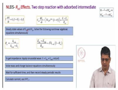
In order to get the steady state value, we say this goes to 0, this goes to 0. We have 2 equations here k1 depends on e2dc. So we have 2 equations to our notes we do not know E2dc and we do not know steady state value of theta. You can solve this. These are 2 algebraic equation non linear equation, but you can solve them and then get the values of E2dc and theta ss use that as the starting point or initial value and integrate these 2 equation simultaneously.
