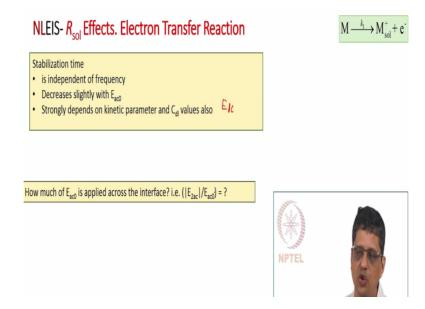
Now how long does it take to stabilize it is independent of frequency. It does vary with Eac 0 and it is strongly depends on the kinetic parameter values, double layer capacitance values and the dc potential at which we acquire the data. Now if I apply an ac potential not all of that falls across the interface a part of it falls across the solution. Now how much of the Eac 0 applied actually falls across the interface.
