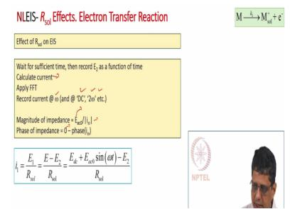
So the way we do this is apply a ac potential wait for some time to get steady periodic response and then in simulations we can record E2 as a function of time. Once you record E2 you can calculate E1 and then calculate the i1 that is basically calculate the current and then apply Fourier Transform mark the current at omega fundamental as well as at 2 omega, 3 omega dc any other frequency you want you can calculate that and record that.
