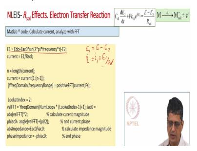
And after you integrate this you can estimate the value of E1 saying E1 is E- E2 current of course is I that is-i1 E1/R solution and then the standard procedure of applying Fourier Transform. So we calculate the impedance at 1 frequency if we repeat it for n number of frequencies we can get the spectral.
