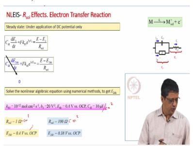
So if I apply dc potential and do not apply any ac potential that means E1 is going to be constant. Constant meaning it is going to be invariant with respect to time E2 is going to be constant. We can say that this goes to 0 dE1/dt goes to 0 and the remaining terms can be solved numerically it is an algebraic equation non linear algebraic equation, but you can solve this and get the value for E2 dc.
