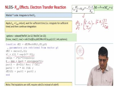
And once you find the E2dc use that as initial value and you have integrate this equation which is basically take this equation rearrange as d E2/dt as E- E2/R solution- F k1 the entire thing/Cdl. So we take the parameter we need to use ode15s because it is a stiff equation we find the value of k1, we write the value of E the first part we write it as E-E2/R solution/Cdl second part we write it as F k1/Cdl and this is the derivative.
