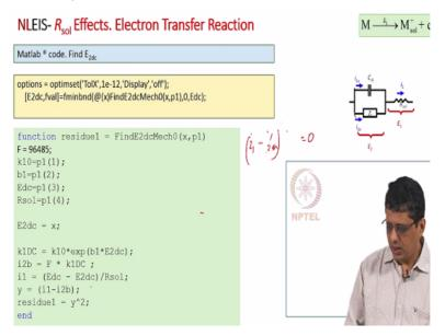
And then first find the dc potential occurring across this interface and we need to give that as the initial value for the integration okay. So in this case I have used the function called fminbnd. So essentially what we do is to take the dc equation which is i1-i2a-i2b=0. I1 is Edc-E2dc/R solution i1b faradaic current is F k1DC and i2a is 0 because when you apply dc potential no current passes through the double layer capacitance.
