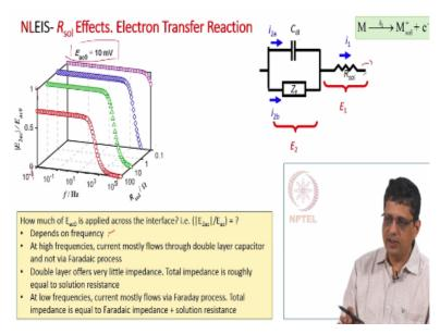
Now we can do the calculation for a variety of solution resistance values and for various frequencies okay for one perturbation amplitude 10 millivolt this is what we see. At low frequencies it is more independent after frequency at high frequency it is very small and at intermediate frequency of course it falls from high value to a low value and ideal value is of course 1. When solution resistance is small pretty across this frequency region it is more or less 1.
