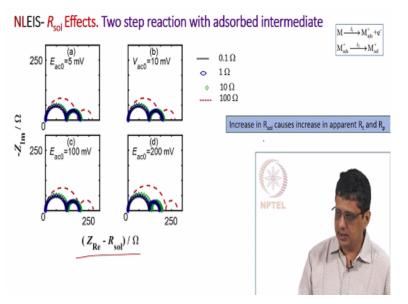
I am not showing you the code I am just showing you the final results this case for this given set of kinetic parameter you get 2 capacitive loops. When you change the solution resistance here it increases, but I also want you to note the following. I have plot a different perturbation amplitude here you can replot it for a given solution resistance different amplitudes and in all cases we have plotted real part of impedance after subtracting the solution resistance.
