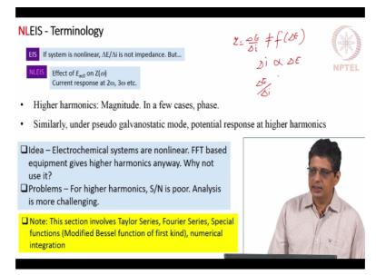
So first impedance is basically the ratio, vector ratio of potential to current, we apply a small amplitude perturbation del E and we monitor the current or change in current del i and that is differential impedance, we normally call it as impedance okay and that ratio of del E/del i that is actually not a function of del E that is the assumption. Del i is proportional to del E that is another way of saying it okay and this is valid if the system is linear.
