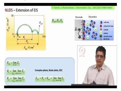
So to refresh your memory, we have seen few terms, solution resistance, charge transfer resistance and polarization resistance. If we take an electrode system, this is one example. If we have a system with one adsorbed intermediate, a clean system with rapid mass transfer, you can get a data like this. This is in complex plane plot, at high frequencies; the total impedance of the system gives us what is called as R solution.
