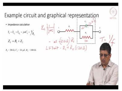
There is a little more complex system where you have 1 resistor in series with another box. That box contains 1 capacitor in parallel with the resistor. I am taking up this circuit because this can be used to model a very simple electrochemical reaction under certain assumptions. We assume mass transfer is very fast. We assume the reaction is very simple, straightforward, one-step reaction.
