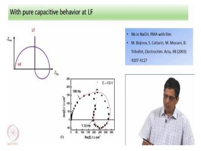
[Please refer to 33.30] And finally I want to show an example where you have high frequency data after normal capacitive data, mid frequency inductive data and at low frequency it behaves pretty much like an ideal capacitor. So it just goes as a vertical line as straight line. This was seen in Niobium dissolving in concentrated NaOH, possibly at elevated temperatures and published by Professor Bojinov and others in 2003.
