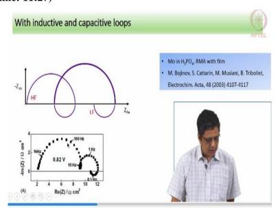
[Please refer to video 11.35] A further extension of this, you have high frequency capacitive, mid frequency inductive followed by a capacitive loop followed by an inductive loop and this has been shown or this has been observed for molybdenum dissolving in very high concentration of phosphoric acid. This was published by Professor Bojinov Acta in 2003 and this is modeled using a film dissolution occurring through a film.
