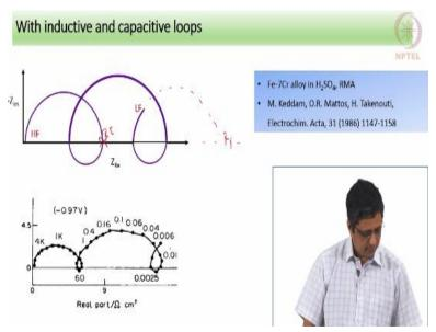
This is a staggering of capacitive loop followed by inductive loop followed by capacitive loop followed by inductive loop followed by capacitive loop again. So this is R<sub>t</sub>, this point
