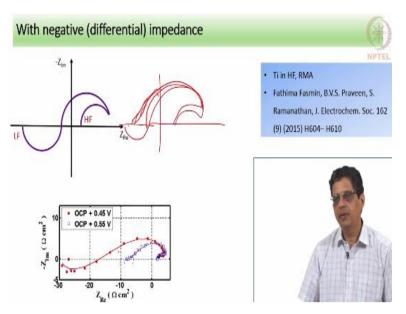
So another way to get the differential resistance, so it is not just going to go to the right side and come back and settle not all the time. [Please refer to video 22.08] You can have a capacitive loop followed by a capacitive loop with negative resistance followed by an inductive loop. So finally it still settles at the negative value. This is seen for Ti dissolving in HF, in the passive region it is published in 2015.
