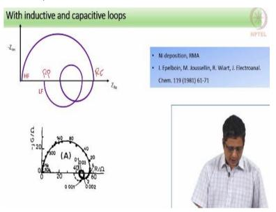
Same set of loops occurring in the same sequence, but with different magnitudes that is capacitive, inductive, capacitive and inductive, but with different magnitudes for these loops or for those inductor values and capacitor values, if we model this with electrical circuit that will give rise to a pattern like this here the polarization resistance is smaller compared to the charge transfer resistance that occur somewhere here, here where I trust the most.
