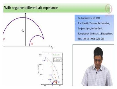
Now I want to show you some examples which give negative impedance, negative impedance meaning, at low frequencies the data settles at the real axis and the value is negative that means  $R_P$  polarization resistance is negative, and we know that it is possible because it is a negative differential impedance it is not negative impedance per se and often we call it as negative resistance.
