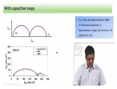
This is one of the simpler ones, of course people have seen data with just a semicircle or part of a semicircle. Here this is an example with two capacitive loops. In all these plots I am going to show you -imaginary on the y axis and real on the x axis., This is a starting point high frequency data and as you go to lower and lower frequencies it forms one capacitive loop followed by a second capacitive loop.
