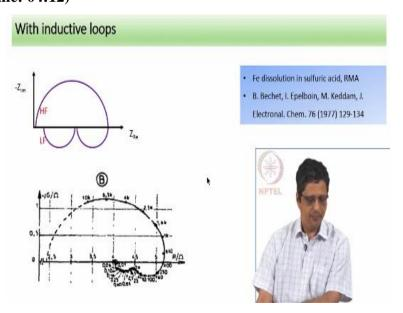
It is possible to have more than one inductive loop. So this starts at high frequency goes to middle frequency, forms one inductive loop and then subsequently it has another inductive loop and this is published in 1977 that means nearly four decades ago. This is ion dissolving in sulfuric acid and this has been analyzed using mechanistic analysis. I do not remember the biased used for this and I do not remember whether it is measured in pseudo galvanostatic mode or pseudo-potentiostatic mode.
