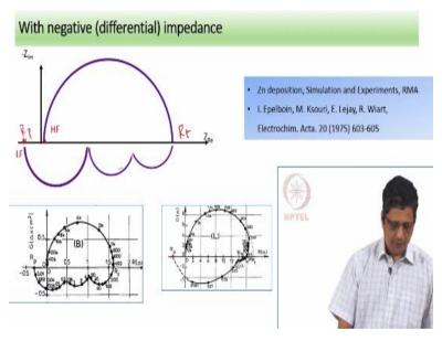
This has been done in simulation when the data of zinc deposition, if I remember right under galvanostatic conditions was analyzed by Professor Epelboin and others published in 1975. In simulations they have seen a high frequency loop here, low frequency inductive loop, second inductive loop and third inductive loop, which still settle at the negative value. In experiments they have taken a data, it has come here one inductive loop is seen here.
