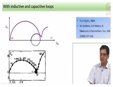
[Please refer to video 16.06] This is capacitive loop at high frequency, inductive loop at mid frequency two capacitive loops at low frequencies. Again seen in iron dissolving in sulfuric acid published in 1981 by Professor Keddam's group and this is analyzed using mechanistic analysis. If you see the actual data you can see the high frequency loop a small inductive loop followed by a small capacitive loop, but before it is completed next capacitive loop manifest here.
