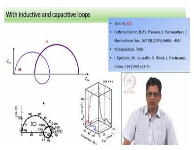
[Please refer to video 9.08] Now inductive loop at low frequencies is the example we have seen before. It is possible to see inductive loop at mid frequency. So capacitive loop followed by an inductive loop followed by a capacitive loop again. This is an example where you have a capacitive loop. It is drawn in 3D plot here so complex plane plot is shown on the red color and the blue color lines are actually form of bode plots where you plot imaginary value of
