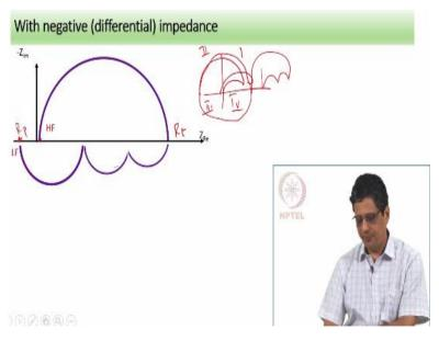
Now negative differential resistance, does not always mean that it has to go on the second quadrant, first, second, third quadrant and fourth quadrant. Many times when we see negative differential resistance actually we do not see negative differential resistance that often compared to a normal data, but the positive regime positive regime, meaning to the right side of this axis.
