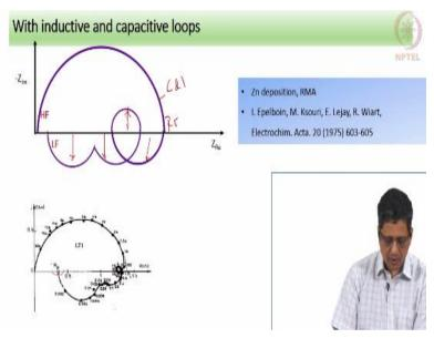
So now this element has three inductive loops and two capacitive loops, that means one high frequency capacitive loop can arise from charge transfer resistance and double layer capacitance. So this we can explain using charge transfer resistance and double layer capacitance and of course this offset is for solution resistance. This is one Maxwell element, this is one Maxwell element and this is one more Maxwell element.
