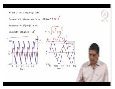
Now I want to give you an example. Let us say the resistance is 1  $\Omega$ . Capacitor is of 0.01 F. We apply a sinusoidal wave of 10 Hz frequency, that means in 1 second you will get 10 complete cycles. There are 2 ways of representing the frequency. F is the normal frequency,  $\omega$  is called angular frequency and that is going to be  $2\pi$  f and that is given in radian per second.
