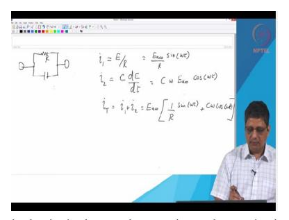
So first we will take the circuit where you have a resistor and a capacitor in parallel. Current through the top part, we will call it as i1 and that is going to be related to the potential applied
