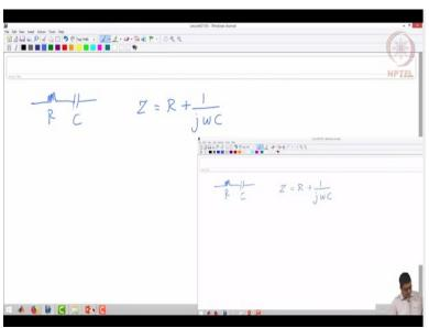
So yesterday, we were looking at this circuit where you have a resistance and capacitance in series and if you write in complex notation, you can easily write the impedance as impedance of resistor and the impedance of the capacitor, add them together, you will get the total impedance. We can write the equation for the current and we have gone through the derivation.
