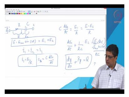
When you actually look at the circuit, it looks very simple and it is simple with R and C connected in series. Now I apply a potential across terminal 1 and terminal 2 and that is given by the value E. We will write it as  $E_{ac0} \sin \omega t$ . The potential drop across the resistor, we call it as  $E_1$  and across the capacitor, we call as  $E_2$  and we can write the total potential drop is going to be sum of  $E_1$  and  $E_2$ , algebraic sum of  $E_1$  and  $E_2$ .
