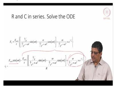
And we can get the potential across the capacitor as  $E_2$ , right. We will get a fairly lengthy expression. The point that I want you to note is that there is an exponential term. We know it is a resistor and capacitor in series. So we know the potential across the capacitor. We can calculate the potential across the resistor.
