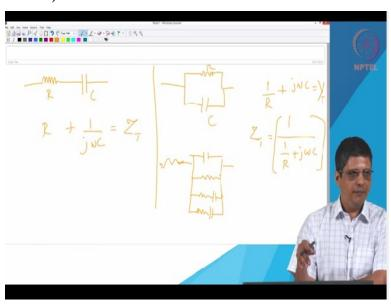
Another example is having resistor and capacitor in parallel. If you look at the second example, it is actually simpler to solve. Previously, I told that you can get the current across the capacitor by
