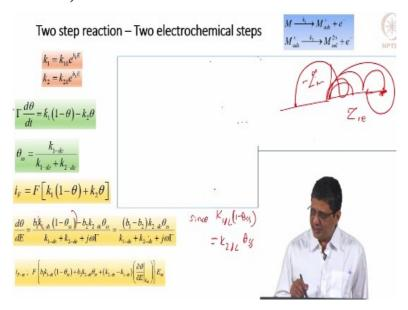
[(refer video, 25:42)  $Z_{\text{real}}$  vs.  $Z_{\text{imaginary}}$  it is called Nyquist plot or complex plane plot, where you have impedance going like this, impedance going like this, impedance going like this, impedance going like this. And it starts at high frequency ends up at low frequency and my
