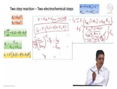
If I want the impedance I should write it as  $E_{ac}/i_{Fac}$  for the faradaic impedance, or I can write the admittance as  $i_{ac}/E_{ac}$ . This as  $i_{dc}$  and  $i_{ac}$  (refer video, 12:35). It is easy to write  $i_{ac}/E_{ac}$ . This term here is the faradaic admittance. As long as I can get this  $d\theta/dE$  correctly, I have an expression for the faradaic admittance, which means I can get the faradaic impedance, therefore, the total impedance.
