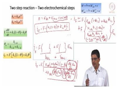
[I am going to say] the potential is  $dc + ac_0 \sin(\omega t)$  and I will use certain approximation.  $k_{1dc}$  multiplied by (refer video, 06:00), likewise  $k_{2dc}$  multiplied by  $E_{ac}$ , where  $E_{ac}$  is the time dependent function here. What this means is, [we look at]  $k_1$  is a function of potential. We write it as  $E_{dc} + E_{ac}$  (and) we expand the  $exp(b_1E_{ac})$  in Taylor series, we truncate it [we go through few steps and then come to this approximation].
