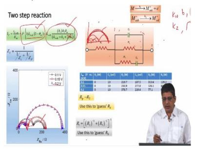
In the last class we saw an example of a reaction two step reaction which is Metal going to Metal<sup>+</sup> adsorbed and then Metal<sup>+</sup> adsorbed going into the solution and then derived the expression for the impedance for this reaction.
