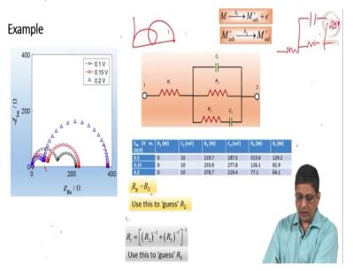
Now, later we will see that if you have a reaction like this, it is possible to get impedance spectrum like this. At different DC voltages, we will get three different spectra here. Now I want to fit it to the circuit. I have two capacitance loops; I am going to use one Maxwell circuit like this. Solution resistance is more or less zero. This is artificial data of course, so I made it as 0. (We should get the double layer capacitance, and all other resistances).
