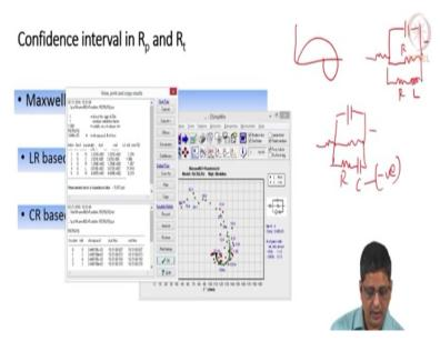
I want you to look at the values of the elements. The resistance, the first resistance here is  $10~\Omega$ , it is  $1.03\times 10^1$ , relative standard error is 1.3%. Capacitor is  $20~\mu F$  that is also coming correctly 2%.  $125~\Omega$ , is the resistance here. So this resistor is  $125~\Omega$ . Standard deviation is 1.4%. That means in this representation, I know at infinite frequency, current will not go through this, so charge transfer resistance here is  $125~\Omega$ .
