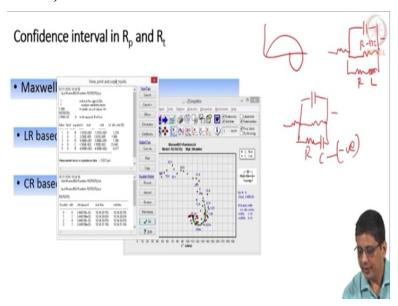
The percentage standard deviation, relative standard deviation is different now. Because of the way that each element is related to the impedance. So you have 23-24% relative standard error for the capacitance. We have 8% standard error in the resistor, which is associated with the capacitor. This value the one associated with  $R_p$ , we have confidence now. So now we have good confidence in the value of  $R_p$ ,  $R_p$  is close to  $100 \Omega$ .
