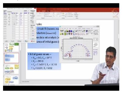
Instead of fitting to the circuit, I used the CRCR. We know that we have 1 inductive loop. We cannot model everything with capacitance. However, a Maxwell pair with negative RC can model an equivalent with positive LR. That is something that you will learn. I leave the original resistance, double layer capacitance, 1 more resistor, then parallel CR as positive, 1 more parallel CR, I keep it as negative.
