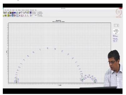
This capacitor and resistor are large values (1.5 mF and 500  $\Omega$ ). Still I can tell that if I use this model, it fits well, no problem.
