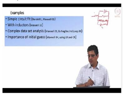
For this, I will use the following circuit (refer video, 12:37). This circuit will give me 1 capacitive loop. This is offset, this is capacitive loop. This element here is an inductor. And this is a resistor. I will use a capacitive loop here. But I also need to know that it will end up in a negative resistance. At the low frequency, it has to end in a negative resistance. (Refer Slide Time: 13:20)
