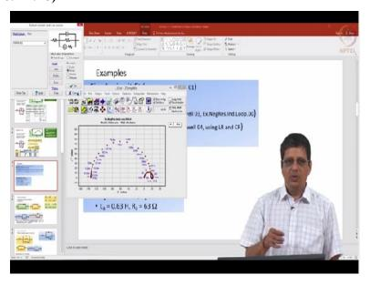
I want to show data which looks like this (refer video, 11:30). That means in the complex plane, it has an inductive loop and a capacitive loop that goes to the negative side. It has 1 capacitive loop at the high frequency. It has 1 inductive loop in the mid frequency. And 1 more capacitive loop except that it is going back.
