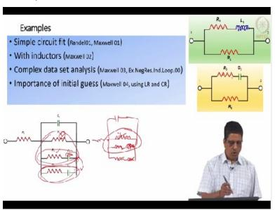
Likewise, if I have a much larger circuit (refer video, 43:01). Look at this Maxwell circuit with resistance, 1 Maxwell pair, second Maxwell pair here. I can replace 1 2 3 with new resistance, resistance, and inductance, that means this will be a new number. This is going to be a different
