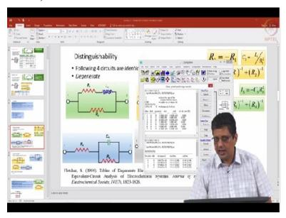
In this case, I will have to take the circuit. I have to take the bottom 2 which is CR which are on the negative region. And I have to take this resistance which is just below the capacitor. what I have is the following.
