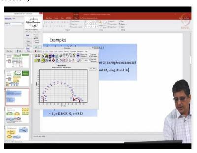
When you look at this, you can see there are 2 semicircles (refer video, 5:56). I can fit it with one more pair of capacitor and resistor. I can arrange it as a Voigt circuit, Ladder circuit, or
