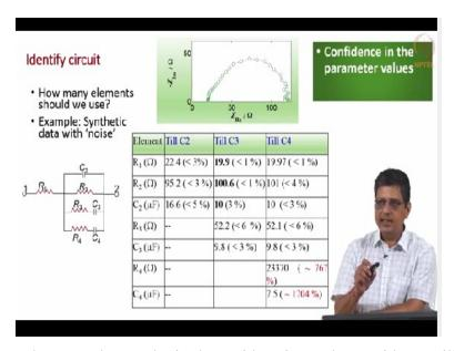
In this example, we have used a synthetic data with noise and we said we will use  $R_1$   $C_2$   $R_2$  in this example. Then we fitted to one more pair of Maxwell element. We look at 2 pairs of Maxwell elements. Confidence interval is poor in  $R_4C_4$  case. We also did estimate of AIC and said, this circuit can be fitted well with  $C_2R_2$ ,  $R_3C_3$  and we do not need  $R_4C_4$ .
