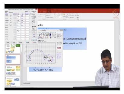
And here also, I am going to use the circuit RCR. RCR for the first loop. Second loop is another CR. Third loop is LR. Except that I do not need negative values anywhere. I can go with the auto setup or I can give initial values. capacitive loop, another capacitive loop, inductive loop, it fits well.
