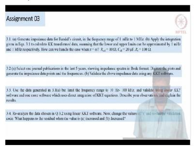
So in today's assignment, I would like you to learn about KKT by doing this homework problem. In the first part,... by now you know what the Randel's circuit is, right? So, (in the) first part, I want you to synthesize the spectrum for a Randel circuit with  $10~\Omega$  of solution resistance,  $20~\mu F$  of double layer capacitance and  $100~\Omega$  for charge transfer resistance. I would like you to synthesize frequencies in the range of 1 mHz through 1 MHz.
