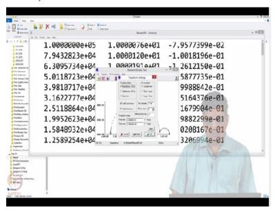
We want to transform this in impedance mode. You can leave *this* checked; if necessary, it will add a capacitor or inductor. This software works only in the *complex test* mode. It does not work (in other modes), for whatever reason. The  $\tau$  value is *time constant per decade*. Default value is 7, you can leave it *as it is*. *This* you do not need to touch; it will look at the data and calculate this.
