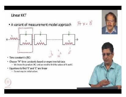
So this is similar to the measurement model that we have discussed before, okay. Except that we want to find  $R_1$   $C_1$   $R_2$   $C_2$  and so on, and (then) see what gives us the best fit. Here, there is an additional constraint. When you look at the circuit, you can calculate the time constant for each of this Voigt element. This entire thing in the box is called Voigt element. It has 1 capacitor and 1 resistor.
