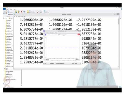
So you say "do KK transform", it will do the transform and tell you the residuals, how they (vary) as a function of frequency. Frequency is from 1 mHz to 100 kHz here. And of course, this is synthesized data. So (residuals are ) at 0; it fits exactly.
