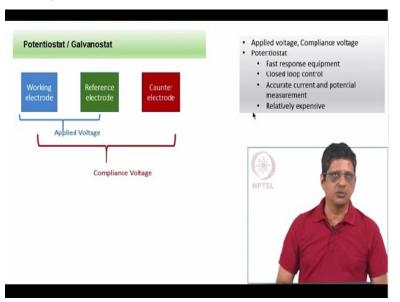
So this is just a pictorial description to tell you what is the applied voltage, where it is measured and what is the compliance voltage, it is measured across the working electrode and the counter electrode.
