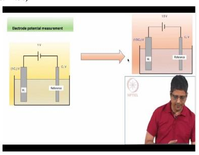
Let us say that  $C_1$  is the potential drop across the metal liquid interface. It usually consists of multiple interfaces. From the metal to the electrolyte liquid, let us say the potential drop is  $C_1$ . It
