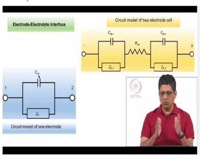
Now if I have one electrode, right next to that is the electrolyte. I have shown that, you can describe that by a capacitor and we call that as a double layer capacitor and we represent that by  $C_{dl}$ . So on the left hand side picture in the blue colour diagram, you have got  $C_{dl}$  but this assumes
