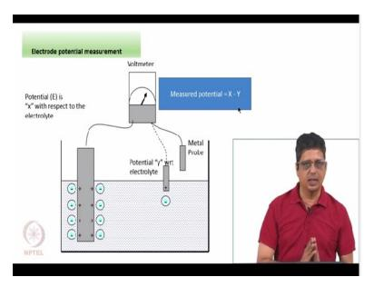
When we put an electrode or a metal in solution, it develops a potential. Can we measure the potential? There is a difficulty associated with that, so I want to describe that here. We cannot measure the potential of a single electrode. The moment we immerse the electrode; it forms a double layer, there is a potential. We want to know the potential difference across the double layer, across the electrode-electrolyte interface. In order to do that, we will connect it to a multimeter.
