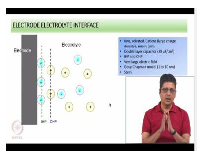
If you imagine, you have metal electrode on one side and water based electrolyte on the other side. The moment we put a metal into the liquid, ions in the liquid will come and adsorb on the metal. So this can be visualized as follows: you have one layer of ions adsorbed on this electrode and that forms what is called inner Helmholtz plane or IHP, that is given by the green colour line here.
