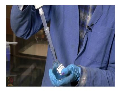
So, now we will take 10 ml of oxalic acid into to this pipette. This 10 ml oxalic acid will now add to this 100 ml conical flask. We will then add few drops of phenolphthalein indicator to it. After adding the phenolphthalein indicator, we will now perform the titration using NAOH.
