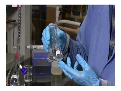
So, now we can see that our solution has changed from colorless to slightly purple color which indicates that the reaction has raised its end point. So, because phenolphthalein is colorless in neutral or acidic condition but it purple in slightly alkaline or alkaline medium. So, because we have added a slight excess of NaOH to determine its end point so, the solution has turned to purple color. And we can see that we started from 0 marker of our burette and we have reached at around 16.8 ml.
