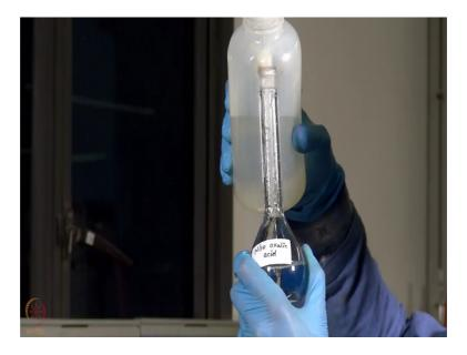
So, now that we have our 0.1 normal oxalic acid prepared which you prepared by adding 0.63 gram of solid oxalic acid dehydrate into 100 ml of water. So, what will we do next? We will take 10 ml of this oxalic acid solution into a 100 ml conical flask.
