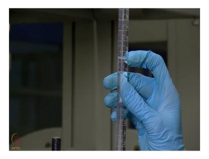
So, 16.8 ml of NaOH is required to neutralize this 0.1, normal 10 ml of 0.1 normal oxalic acid solution. Now, you will repeat this experiment two more times to get concode and tradings. We will then average these readings for our further calculations. So, now, that our standard calculation of NaOH is complete. We will now standardize our HCL using tis NaOH. We will take 5 ml of HCL into this conical flask and then add phenolphthalein indicator to it.
