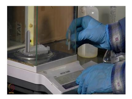
So, we will now weigh 0.63 gram of oxalic acid dihydrate. So, we have now around 0.63 gram of oxalic acid we will take it out and we will then add it to a 100 ml volumetric flask.
