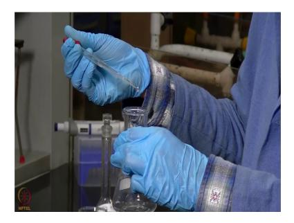
And we will now titrate it using NaOH. So, now, the titration of our HCL is complete. Now, we will perform this experiment two more times and try to get concordant readings and then we will use these readings for our calculation. Now, that we have standardized our NaOH and HCL solutions will be taking 50 ml of the HCL solution that we had prepared in this conical flask. And then we will be adding 2 ml of methyl acetate to it.
