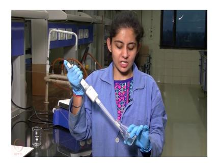
This is the methyl acetate and HCL mixture that we had. So, we will be withdrawing 10 ml from the solution. And will be putting it inside a beaker then will heat on a heating mantle at 70 degree celsius for half an hour.
