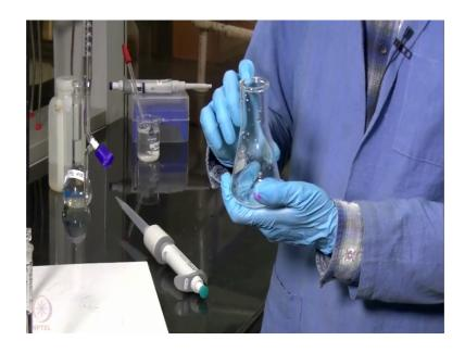
And we will then add phenolphthalein to it as an indicator. So, we know that under basic condition phenolphthalein changes its color from colorless to pink color or purple color which shows that indication of the reaction that the reaction is completed.
