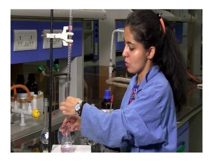
Now that the titration is complete and the color of solution has changed to purple. The value that we are getting here corresponds to the V naught value that will be using for further calculation. Now similarly, we will be titrating the solution which we have kept at different intervals of time will be withdrawing the solutions and titrating in a similar manner and will proceed.
