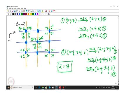
What does it mean? We have a C centred lattice, then we have a mirror perpendicular to x a mirror perpendicular to y and a twofold parallel to z so now for my easy understanding, I am making the rectangular divided into four parts because I need to
