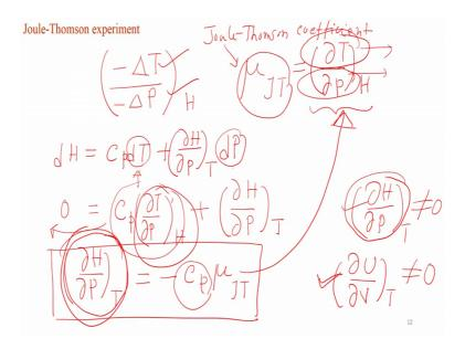
So, what joule and Thomson measured is the associated temperature drop which is minus delta T as a function of the associated drop in pressure at a constant enthalpy. So, they defined a term which they called as mu J T which is known as the Joule Thomson coefficient and defined it at the change in temperature as a function of pressure for a constant enthalpy process which was carried out in there or measured in their experiment now what will be the expression of del T del P H.
