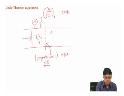
When Joule and Thomson carried out another experiment which is known as Joule Thomson experiment they figured out that there is a small, but finite change in that quantity del H del p t. So, Joule Thomson experiment discusses about measuring this quantity del H del p T experimentally. Now let us first describe what is the experiment, in this experiment Joule Thomson took a cell tube and inside the cell tube there was a wall which is a perforated wall.
