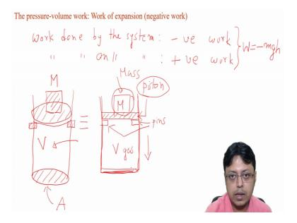
Now again remember that the convention is if the work is done by the system, then we will call it as a negative work and if work is done on the system by the surroundings then we will call it as a positive work and for that we asserted that the definition of the world in the definition of the work we have to insert a negative sign.
