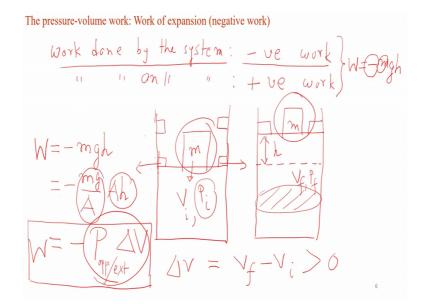
Now think about it suppose initially suppose this is our system and this is the piston and then we have kept a mass on it and suppose the pins are connected like this in this case the pressure inside this pressure of this gas, which we denote as say P i i is for initial pressure and the associated falling mass V i the pressure is enough to raise this mass which we denoted as M, we have been using the mass as small m. So, let us just write it as small m instead of capital M.
