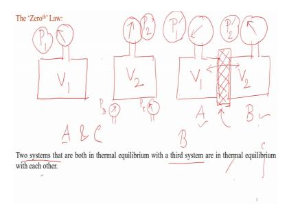
So, the Zeroth law says 2 systems that are both in thermal equilibrium these 2 systems which chose remember as A and C the 2 systems, which are in which are both in thermal equilibrium with a third system which is chose as B are in thermal equilibrium with each other which means A and C are also in thermal equilibrium.
