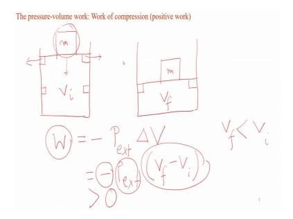
So, in the case of compression we have a opposite situation. So, initially suppose the volume was vi according to our convention and then it was the piston was held by 2 pins and there was a mass now of course, this mass is creating more pressure that is why if we remove the spins the mass will fall and let us put 2 more pins so, that the piston will fall up to a certain height.
