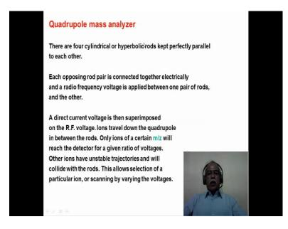
Now, let us have a look at the quadrupole analyser. A quadrupole is a quadruply charged system. And, there are 4 cylindrical or hyperbolic rod, which are kept in parallel; kept parallel to each other. Each opposing rod is connected to an electrically as well as radio frequency voltage that is applied between a pair of electrodes.
