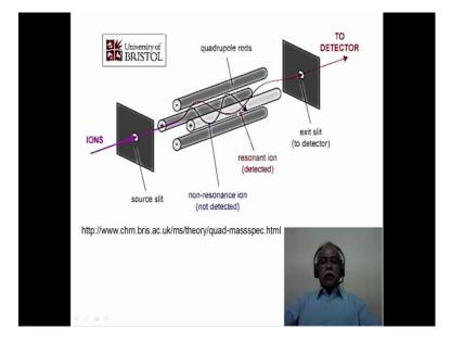
This is better explained using a diagram like this, for example. These 4 poles that are shown here are the quadrupoles of this type. And, the quadrupole has the opposite, the adjacent quadrupolar rods have the opposite polarity; plus minus, plus and minus. So,
