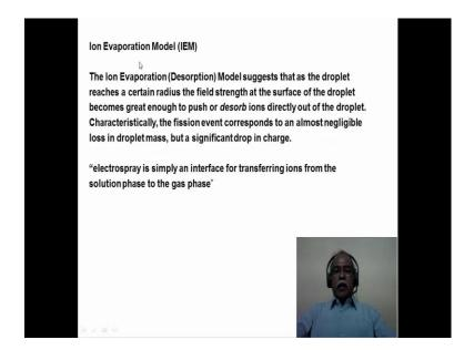
In the case of, the Ion Evaporation Model, as the radius of the droplets becomes smaller and smaller, the field strength at the surface of the droplet becomes enormous. And, that directly pushes the ions out of the droplets. So, this is ion evaporation model. It is slightly different from the earlier model. Essentially, the electrospray ionization is simply an interface for transferring ions from the solution phase into the gas phase. If you look at the mechanism by which they undergo this.
