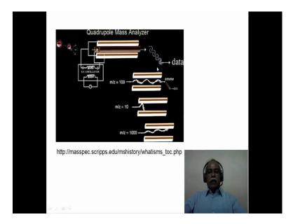
This is given in another diagrammatic representation here, for example, this is a quadrupolar analyzer. For example, in this particular case, there are 3 ions m by z of 10, m by z of 1000 and m by z of 100. The applied voltage is such that only the m by z value of 100 passes through the; this is called the resonant ion, which passes through the quadrupole analyzer to the detector.
