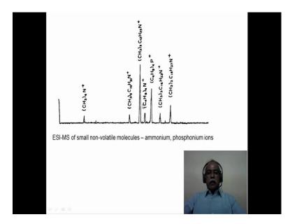
Now, this is a mass spectrum of certain non-volatile molecules. These are actually ammonium and phosphonium ions. This is tetrabutylammonium bromide or ammonium iodide. Please, remember that when you do a positive ion mass spectrometry, only the positive ions will be detected. The counter ion as it may be chloride or bromide; it is not going to be detected in the mass spectrum. So, this is a positive ion mass spectrum; is of the various ions is shown. These are all non-volatile ionic substances.
