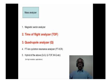
Typically, the electrospray ionisation mass spectrometry with the quadrupole analyser and the time of flight analyser, what we call as the Q-TOF ESI is a standard combination. Whereas, in the case of MALDI, MALDI-TOF is the standard combination; where MALDI is the ionization methodology and the time of flight analyser is the mass analyser as a standard combination.
