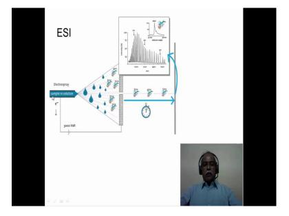
Now, in the electrospray ionization mass spectrometer, there is an injector which sprays the solution or the analyte to be analysed in the form of very fine droplets. And, it does so in a voltage region, where the sprayer itself is a one electrode and there is a counter electrode which is kept here. And during the course of the fine spray, there is also a nebulising gas which is passed through the sample. This is better represented in the next slide.
