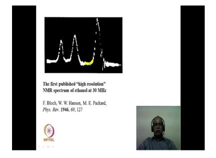
Now, here the very first spectrum of ethyl alcohol published using a 30 megahertz NMR spectrometer corresponding to roughly 0.7 Tesla of magnetic field strength. This is a very unresolved spectrum in today's standard; nevertheless, from the historic perspective it is the very important discovery. Now, when we look at the spectrum you see three different peaks in the NMR spectrum and if you look at the structure of a ethyl alcohol there is CH
