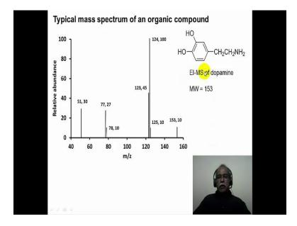
In this particular example, the ion is generated by removing an electron from this molecule. In other words, by the ionization of this molecule and the cat ion radical thus produced is the one that is responsible for all the other ions that are produced. So, essentially, the removal of an electron is what we are calling as ionization process in this particular technique. It is not always necessary to remove an electron, one can always
