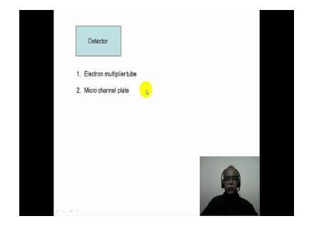
Now, the detectors are essentially electron multiplier tubes or micro channel plate. The ions impinge on these electron multiplier tubes and produce a current and the current is what is registered as a signal corresponding to the mass spectrum that one records.
