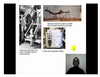
These are some pictures of mass spectrometers. The very early mass spectrometer is shown here. The one that is developed by J. J. Thompson, this is a replica of that. Here you have the ionization chamber where the substrate is reduced and ionized. It is passed on to an accelerator chamber where they are given a certain kinetic energy to travel and then, they enter the magnetic sector analyzer. This is the magnetic sector analyzer.
