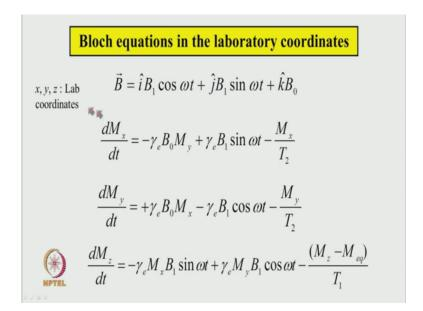
Then the total magnetic field that the magnetization experiences due to the external magnetic field B 0, and the oscillating magnetic field B 1 cos omega T in the x component, B 1 sin omega T is a y component total magnetic field. Then we get these 3 equations. And here this x small x small y, and small z these are the laboratory fixed x y z coordinate any particular the B 0 the Zeeman field is applied along the z direction.
