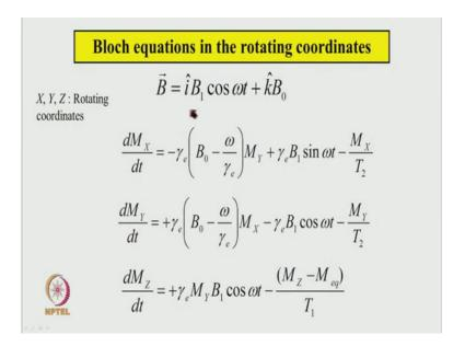
So, that capital x y and z are the rotating coordinate system. Then are the total magnetic field appears only as a x component of the (Refer Time: 33:52) and the Zeeman field is around the y, I am sorry in the z direction, and then this time dependence of the x y and z direction.
