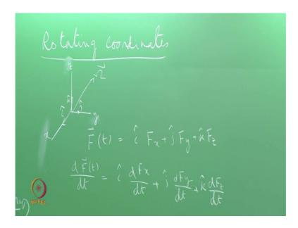
Suppose I have got a coordinate system, let us call it capital x y and z, and this is rotating in a certain direction may be let us I have say I have got this capital x and y and z a coordinate system, which is rotating about an axis at a certain angular velocity omega.
