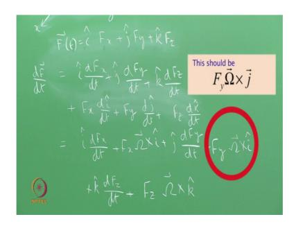
So, this will be f of x di by dt plus f of y d j by dt and plus f of z d k by dt. So, this gives the complete time derivative where coordinate system is also rotating.
