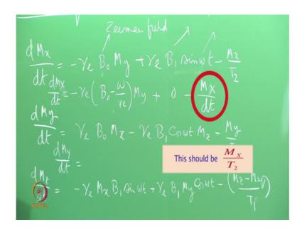
These things indicate that this is the rotating coordinate system. Similarly, for y component dM y by dt will be B 0 will be replaced by this one.
