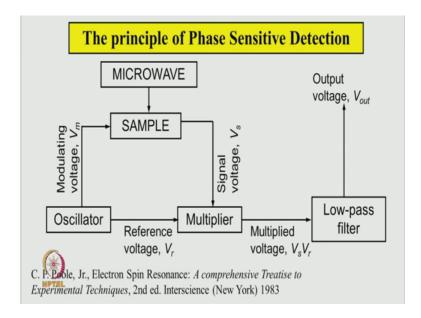
Here, let us say micro comes from this place and falls on the sample and microwave is absorbed by the sample and is producing a signal which comes out here in the form of signal voltage.
