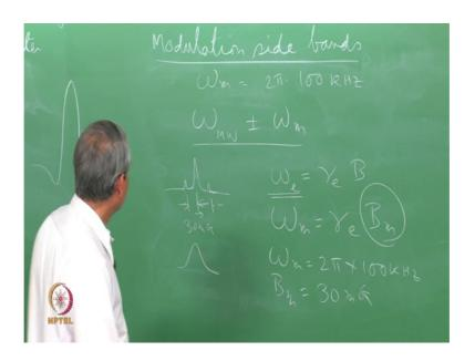
So, here we are using some ac modulation of the order of less typically 100 kilohertz. So, omega of modulation is a 2 pi times 100 kilohertz. So, this frequency is causing the magnetic field to be modulated. So, a here the diode sees a signal that comes out of cavity which is getting modulated with this frequency. So, this will be generating as
