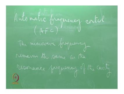
So, that technique is called the automatic frequency control. First of all, AFC, it is job is to ensure that the microwave frequency remains the same as the resonance frequency of the cavity. And this has to be done one extended period of time. How is it done? To understand that it is again recall how the cavity responds to change in the frequency of microwave.
