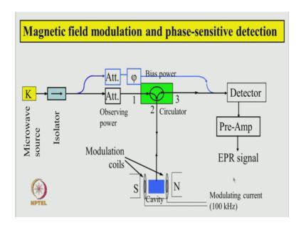
What is done is shown here, that we modulate the magnetic field that Zeeman magnetic field are here by using a pair of Helmholtz coil, which is mounted easily on the cavity. This this modulating current is passed through this coil typically at 100 kilo hertz; so the main magnetic field, which is the Zeeman magnetic field that is modulated at this frequency. What happens then?
