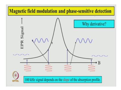
So, the amplitude of this signal depends on the slope of this absorption profile. So, longer this amplitude of modulation are very large. And also, the phase of depends on the whether it is left side or right side.
