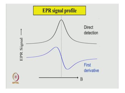
So, there will not be any 100-kilo hertz component here. So, the signal will therefore, look like this. So, this black curve shows the direct detection EPR signal absorption profile, and the first derivative signal will be having this set of profile here, goes up and
