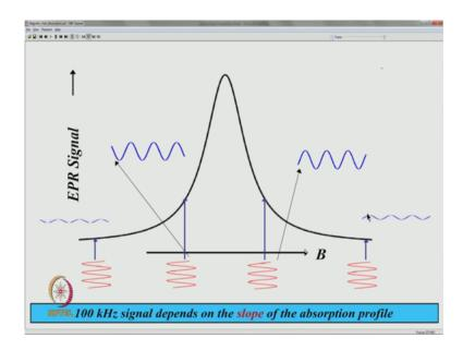
So, a magnetically modulation is shown as red, and the output signal is shown in the blue color at different places of the Zeeman magnetic field. You notice here the phase of this
