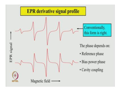
But what will be the ultimate appearance of the EPR spectrum? I said the phase changes through the peak of this thing. So, the absorption profile could be either this way first it goes up comes down, and goes up or comes down. Or it could be first goes down and then comes up or goes down or comes up. What does depend on? Now of course, depends on the reference phase first for here for example.
