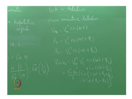
Let us say V m is the modulating voltage, which is let us say V m 0 cos omega t, with the frequency of modulation. V r is the reference voltage that goes to the multiplier, let us call it V r 0 cos omega t plus phi r. And the signal that the sample gives V s similarly, V s 0 is a cos omega t plus phi of signal.
