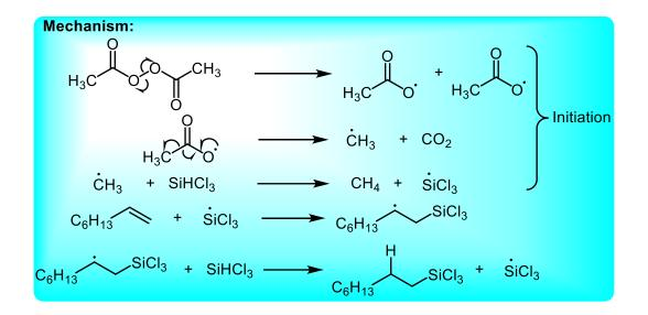
You can see because of this you have this type of the peroxide linkage here which is going to get cleaved in case of heating to generate CH3COO radical after the CO<sub>2</sub> getting eliminated it can form CH<sub>3</sub> radical which can able to form this corresponding silicon radical here.
