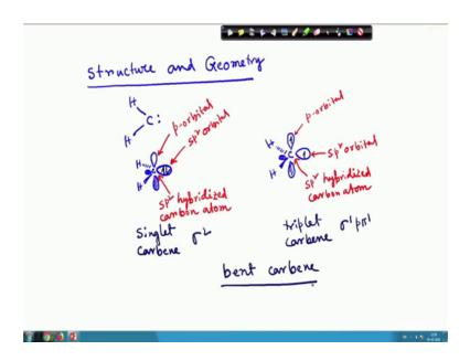
So, our the next topic that will be discussed that is the structure and geometry of the carbenes. First we will see this is the carbenes, now we will draw its structure and geometry ok. So, this is the sp 2 hybridized carbon atom ok. And this is the p orbital ok, and this is the sp 2 orbital ok.
