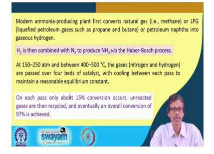
So, the modern ammonia producing plant basically first converts the natural gas that is methane, we have seen that we can have the coal bed methane also. So, methane from that particular methane, we have to extract the corresponding amount of hydrogen, and that hydrogen can be utilized for its reaction with the nitrogen. So, natural gas LPG petroleum naphtha can be utilized for the production of large amount of hydrogen that we have seen also in case of hydrogen production.
