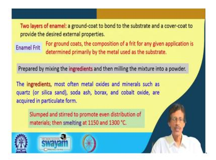
So, a ground coat to bound to the enamel and the cover coat to provide the desired external properties, because ultimately what we will be looking for is the surface. After enamel coating how the surface will look like and how it will be useful for different useful purposes?
