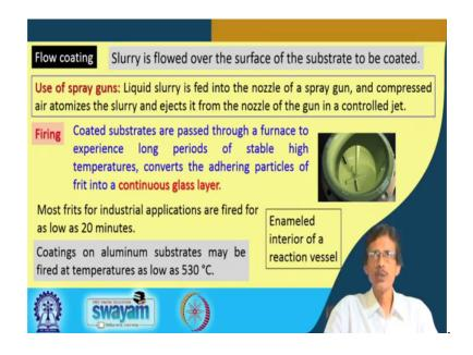
Then, we can have the flow coating also another particular coating; that means what we have seen we have seen that the slurry you can have. So, the liquid you have on the liquid you have the powder material the slurry, and if you want to flow basically the way we spraying the dry material in the similar fashion we can have the flow of that particular material which is in suspension.
