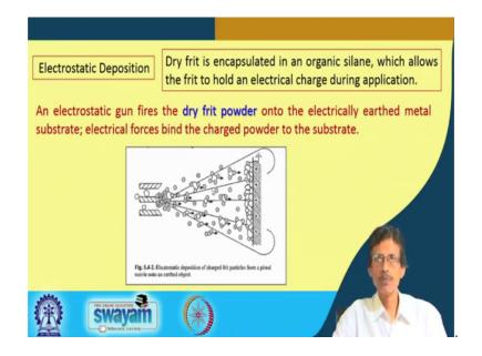
Then, another technique out of this wet and dry application is by using electrostatic deposition. If, we have something where you can have the difficulty in applying these things, through this wet application and dry applications, we can go for electrostatic deposition. So, we will take their particular charged particles. So, we have the particles which are in the powder form like that of your talcum powder, but now if we are able to apply some electric charge such that particles are charged.
