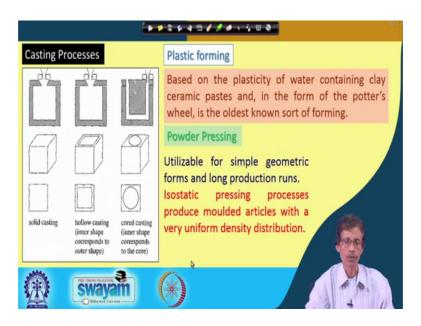
Then, after this forming process we will just proceed for the casting process, we know that the typical the casting how we cast a particular type of material? So, it is also true for your ceramic material. So, we can have a good particular type of mould, or particular type of template in our hand, and the casting is being done of three different categories.
