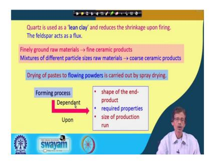
So, if we use this quartz material why we are use these the quartz is use basically as a lean clay, because this is a basically a clay material and we are putting some amount of quartz in it which is nothing, but your S i O 2 material. So, this S i O 2 material and is the purpose of this is that reduces the shrinkage upon firing. So, when we fire it the material is will be fired.
