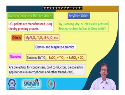
So, the zirconium oxide ceramic can also be utilized, then we can have the uranium oxide or thorium oxide based specialty ceramic material. So, that basically can give us using that uranium O 2; that means, U O 2 pallet us and a manufactured using the dry pressing process. So, in that particular process the dry processing pressing process is giving you the only another variety or specialty variety of that uranium based or the thorium based material.
