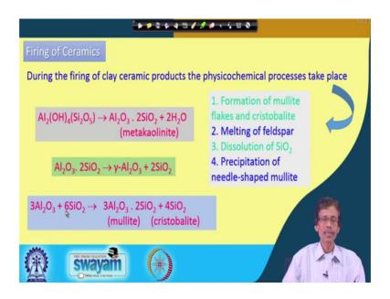
So, once we have this material we have this moulded one like that of your the potters make the different earthenware pots for us and that is when introduced for the typical firing process. And in that particular firing process what we get there is that your typical firing of the ceramics.
