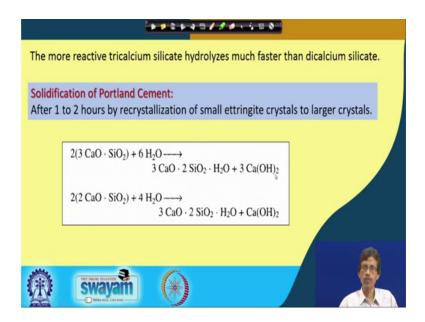
So, next we will find that if you have a tri calcium silicate, which is more reactive and hydrolyzes much faster than dicalcium silicate. So, the rate of the reaction so, these two material are; obviously, different the tri one.
