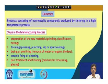
Now, with this we can move to the material, which is known as your ceramic material. So, the ceramics what how with that the difference? So, another important building material or industrially very important material is our ceramics. So, the ceramic industry we have then ceramic engineering we study also so, what are the corresponding basic inorganic chemistry involved in it.
