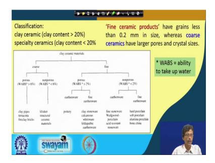
Then, if we classify these materials in terms of two types; one is your clay ceramic which can be considered as the corresponding component as the clay component, we all know this is also a very cheap component. So, when the clay component is above 20 percent, we consider this as only the ceramic made of clay material; that means, is that clay ceramics.
