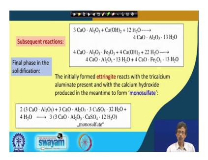
Then, we see that, there will be some subsequent reaction; that means, the further reactions can take place once your tri calcium silicate and di calcium silicate are reacting with the water molecules. So, what are those for the reaction because already we are producing some amount of calcium hydroxide out of that. So, if your now your tri calcium aluminate.
