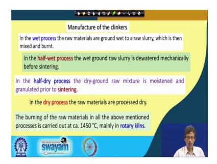
So, next at the end of this particular class or we will continue it in the next that how you get these particular clinkers. So, manufacture of the clinker, so what we get in the wet process the raw materials are making a powder or ground weight to a raw slurry, so when you is in the wet process; that means, the water is there. So, what we get? So, in the
