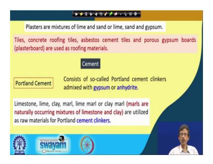
So, then once you get that particular type of concrete you have to have the corresponding plaster because the we cannot expose the concrete to the corresponding moisture, to the corresponding environment because the environment will degrade that particular thing that will not be very much stable. So, what we get? We get some coating agent.
