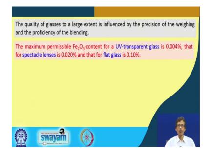
And during that particular process the quality of the glasses to a large extent is influenced by the precision of the weighing and the proficiency of the blending, what type of blending we go and what are the corresponding ratios basically will be using for that particular blending process. So, is basically nothing, but a mixture at a high temperature mixing and blending will give you this particular glass material.
