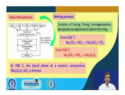
So, this glass manufacture that way is a very important one where we can have the corresponding sand, soda, lime, fled spar and the different types of additive. So, we can have a batch house where we mix all together and all of them is getting when you have a typical homogenized mixture. So, homogenization process we can call, then we put simply put at a very high temperature reactor.
