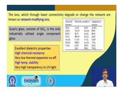
So, these network formers as well as one other variety will be calling as network modifying ions what are those ions? The ions which through lower connectivity degrade or change the network; that means, silicon can have a particular connectivity which equals to 4; that means, can have 4 oxygen surrounding that particular silicon. But if we go to use that particular other methods the other ions based on boron or aluminum, what
