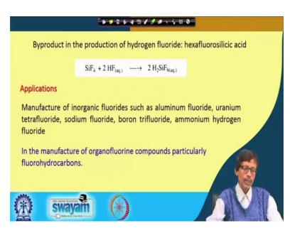
So, this heating procedure is basically giving us the corresponding production of your hydrofluoric acid. And the by product in this production of hydrofluoric acid is that if you have as I told you that you use silica or quartz for taking up your HF production for its conversion to silicon tetrafluoride or H 2 Si F 6, but sometime your silica Si O 2 is already present in your fluorspar, your quality of flora spar is not so good that it has already silicon dioxide or the silica material in it.
