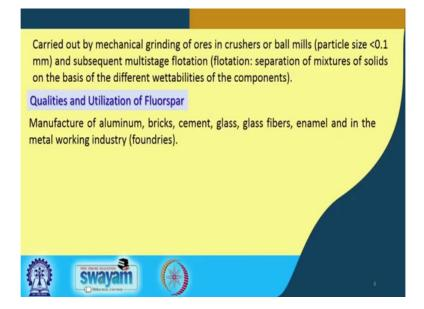
So, is basically carried out, how you do this particular separation or the concentration; is carried out by mechanical grinding. So, mechanically you crush it. So, mechanical grinding of the ores in crusher or ball mills, we know all the what is ball mill and the particle size less than 0.1 millimetre should be achieved and subsequent multistage flotation.
