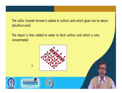
So, the sulfur trioxide formed over there now is added to water and if we add to water that particular sulfur trioxide we get sulfuric acid, but if we add that particular 1 to the formed H 2 S O 4; that means, H 2 S O 4 plus SO 3.
