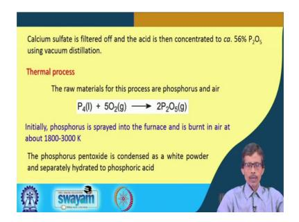
So, it can be filtered off, so calcium sulfate is separated out and the acid is then concentrated to about 56 percent of the actual P 2 O 5, what is known as the corresponding anhydride of your phosphoric acid.
