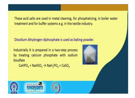
So, how it looks like? One such example I am giving over here is your monosodium, once we call is monosodium phosphate or you can consider as sodium dihydrogen phosphate or Na H2 PO 4. How we make it industrially it is prepared in a 2 step process by treating calcium phosphate with sodium bisulfate.
