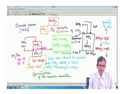
So, the production of nitric acid; as we have already seen that how we can convert your N H 3 to N O, that means nitric oxide formation and that nitric oxide formation is useful for giving you your hydroxyl amine formation. So, what we will see now that this particular nitric acid production this will be dependent on so many things. And one of the thing that we can consider is the corresponding readily available or cheaply available ammonia if we can think of.
