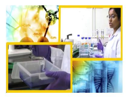
So, this is coomassie brilliant blue which will stain our protein from just pouring the staining solution here closing this and now we will keep this in a rocking motion for almost 1 hour. You can keep it overnight as well and after that we will pour out the stating solution and pour the destining solution.
