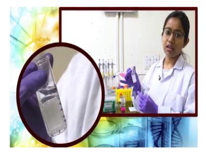
And I have collected all the fractions starting from 18 to 24. So, there was almost 15 ml of solution and using this particular centricon, I have centrifuge this those solution and concentrated the sample.
