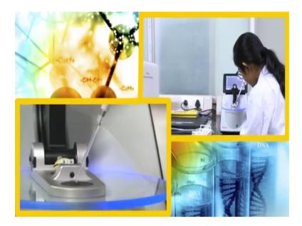
Now, I will load my sample again I am taking two micro liter of the sample and carefully I will load. Try not to make any bubble in that particular small sample, otherwise the absorption will be different and then I will load the blank.
