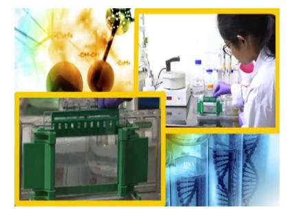
And we will assemble the glass plates to caster gel. So, there is a bigger plate and also smaller shorter plate and this needs to be assembled in a gel caster.
