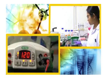
Otherwise you can keep it 100 and run it for a longer time at the same as same rate. Otherwise after the side passed through the stacking gel, you can increase the voltage to save your time. So, we will run till it goes at least half way through the gel and then we will stop and then will put it in this stain.
