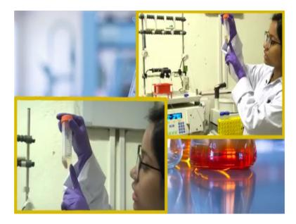
So, our centrifugation has been done and you can clearly see there is the supernatant and the pellet fraction. So, right now, after the centrifugation is over we will separate the solution fraction this will be can the solution fraction.
