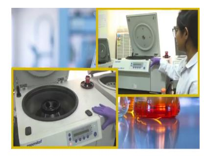
So, we will use a big centrifugation, centrifuge machine for this and this is a high speed rotor. So, this machine can also have basically a low speed rotor also as a high speed rotor.
