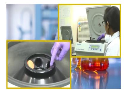
So, put this sample and the weight balance basically at the opposite side. So, it should be exactly opposite, close the rotor head and we will start the centrifugation.
