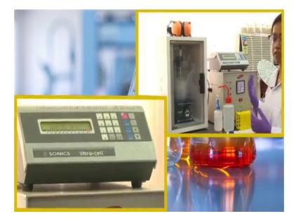
So, in a particular sonicator machine basically you have a cell system, where you can choose the pulses and the amplitude at particular which the vibration will occur, as well as you have a probe.
