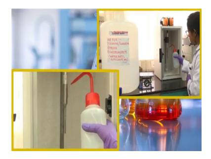
Then we will clean it with deionized water or double autoclaved water. We can wipe it with the tissue paper. So, now, the probe has been cleaned and it is ready to use.
