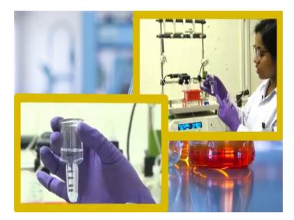
So, along with this falcon tube it has a small holder like this, and this you can see there is a white patch this has the membrane. So, this has a cut off of 3000 Dalton. So, basically what it does is. So, you can see there is written 3000 MCM WCO (Refer Time: 59:16);
