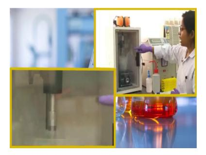
So, there will be a buzz noise coming out from this solution. So, basically it is generating the vibration right now. So, it is on and I have put it for 25 minutes.
