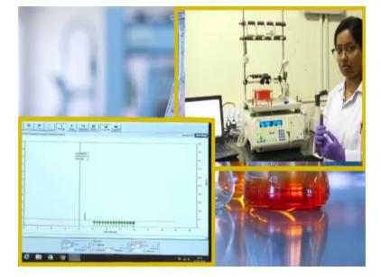
And everything what is happening we can monitor it in this LP date of view basically it will show what is happening. How we can see what is happening? Basically, when the any sample or any solution is passing through this column it will come out from this particular tubing and it will go here. So, this is UV light chamber. So, it will measure the absorbance at 280 nano meter.
