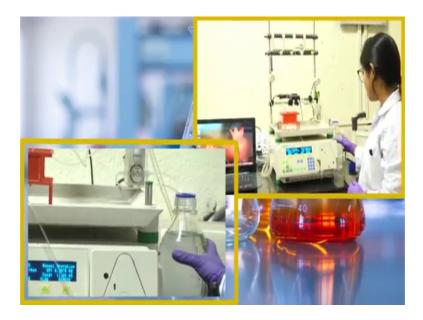
So, in this particular machine we have 2 tubes, buffer A and B in a particular beaker or the container which has only the deionized water.
