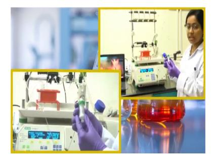
So, this is the Ni NTA column which has this nickel basically beads that are attached to this NTA or the agarose beads. So, while the centrifugation is happening. So, we will make the preparation for our next step. So, in our case our protein is a 6 X histidine tag; basically, it has a 6 consecutive histidine molecules at the in terminal of the protein. So, we can easily separate that particular protein from other cellular components or other proteins. So, we will use Ni NTA a column.
