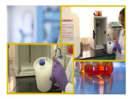
So, for that purpose we will keep over sample solution inside this ice box. So, basically it is inside the ice box. So, and the probe will go inside this solution. So, we will open this cap and it will go inside the solution. So, whenever the heat has been is will be generated and it will be lost because we are keeping it in the ice.
