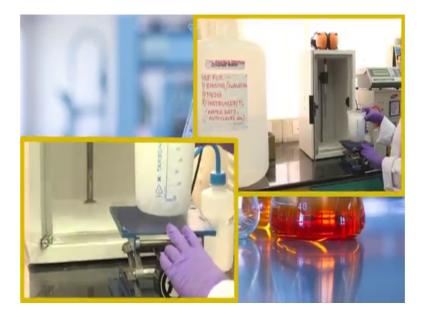
So, there is other in some instrument this is a platform and on the top of which we will keep our sample. So, as you can see in a beaker I have taken amount of ice basically where we use the sonicator, when it generates the ultrasonic sound it vibrates and it creates and heat. So, a large amount of heat has been will be generated and you do not want your sample to be degraded, because proteins are heat labile.
