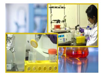
So, this has this filter membrane and in a clean tube you just take that. So, basically it will filter out any kind of particulate matter. There are beyond 0.22 micron. So, this will ensure our longer storage or a longer life time for your column; do not load any crude sample just right away to the column. Now, this is our filtered solution and we will run pass this solution to the column.
