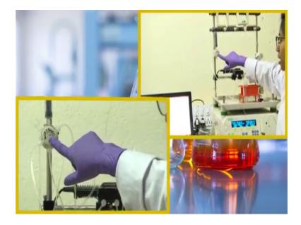
So, this is the syringe fill; that means, it has a mark of syringe. So, basically now you can here in this particular channel you can load your sample. So, before loading I will take my sample in this syringe again. So, this is the filtered sample, if you have any kind of bubbles try to remove the bubbles.
